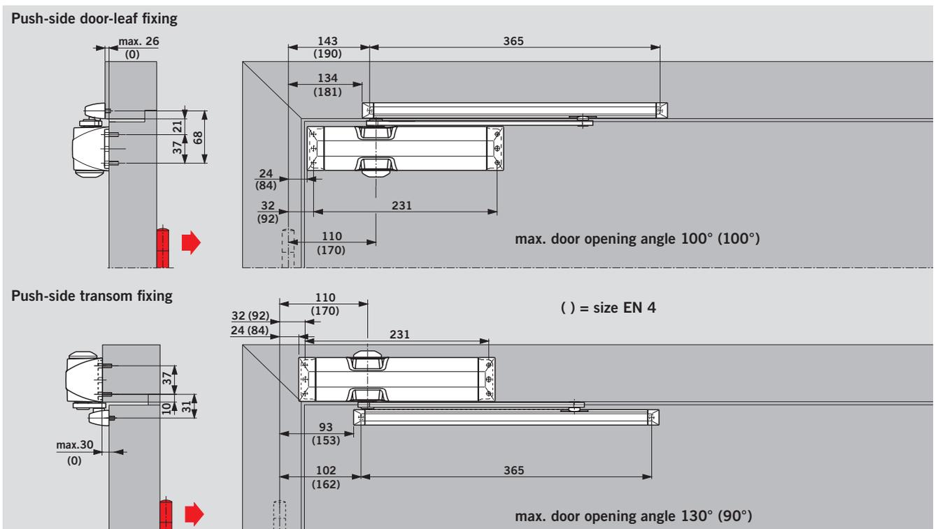
Depending on the structural conditions, the door opening angle is likely to be limited. It is recommended to install the cushioned limit stay or position a door stop at this point.
