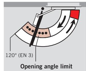
Cushioned limit stay for retrofitting by insertion in the slide channel. Adjustable between 80° and max. 120°.
