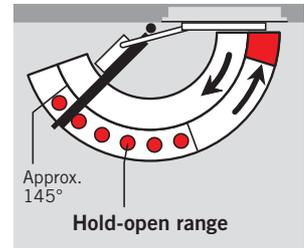
The hold-open device enables doors to be precisely held without any fall-back up to an opening angle of approx. 145°.
